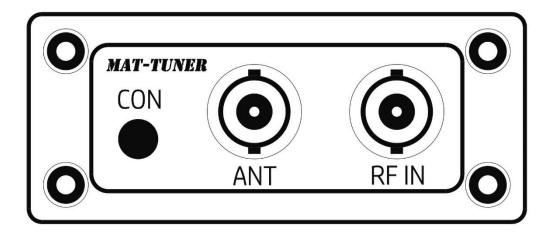
BNC RF socket: There are two BNC RF sockets on the rear panel, they are "ANT" and "RF IN". "ANT" is connected to the antenna. "RF IN" is connected to the ANT socket of the transmitter via a coaxial cable. The coaxial cable mAT-705-RC1 connecting the tuner "RF IN" and the transmitter ANT is not a standard accessory, it is optional.
